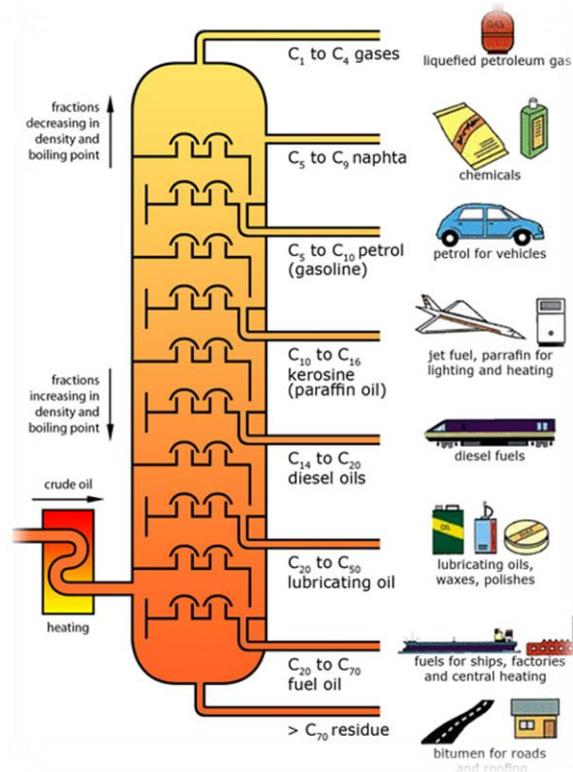
first and are called the heads. The rest of the molecules separate out according to their boiling and condensation points. The heavier, less volatile products settle out and are called the tails. The heart cuts are the gasses that fall between the volatility and boiling point ranges of the heads and tails.
